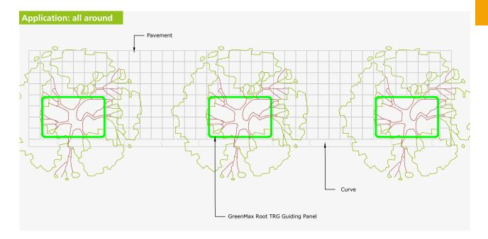
GreenMax TRG Tree Root Guiding is a barrier to control and guide tree roots. Adjacent to services or next to the tree without having to compromise on the health or growth of the tree. TRG can be used for existing and new planting applications.
