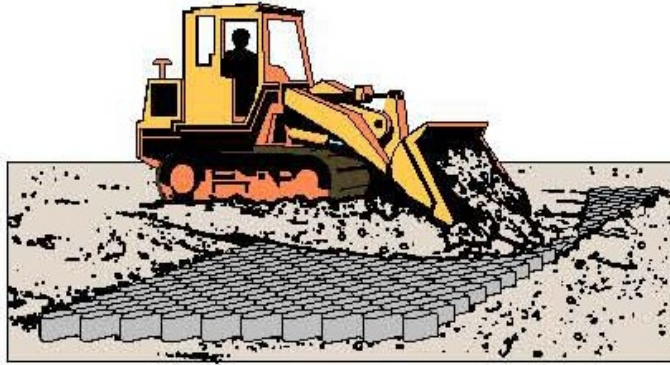
Figure 13 Fill placement with loader
